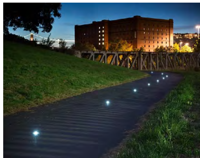
Low level solar studs should be considered where possible (ref: Solareye)
