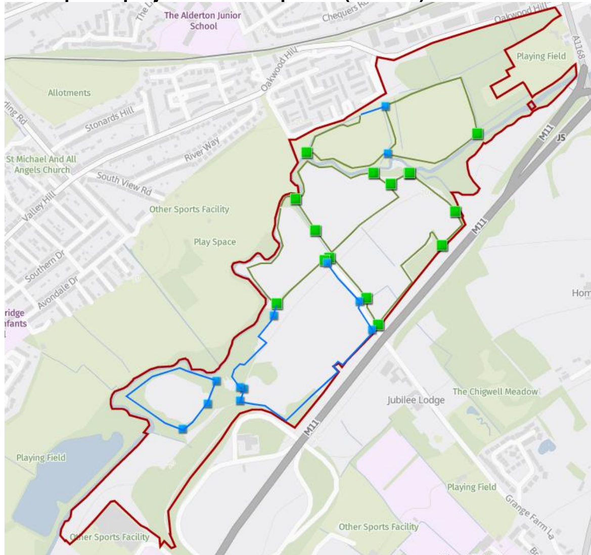
Figure 21 Fencing project 2021. Green: existing livestock fencing and gates, Blue: planned new fencing and gates. Lines: Fence, Squares: Gates
