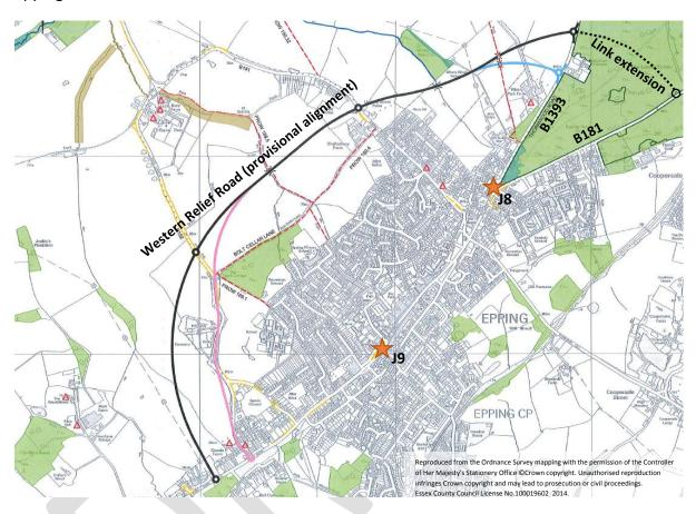
With the relief road and extension in place, there is *potential* for the signalised junction along Thornwood Road to operate largely within capacity in 2036 with no alterations to the junction (other than signal optimisation) required. Although the junction is modelled to exceed capacity under the 'Ambitious Growth A' scenario, PM peak period congestion at the junction is shown to be less than that modelled with 2013 traffic flows.
