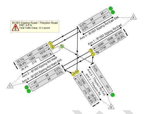
**Evaluation:** The capacity enhancements detailed above allow the Theydon Road signalised junction to operate within capacity under the 'Ambitious Growth C' scenario with a high quota of development in and around Epping. Modelling of the other scenarios suggests that with lower volumes of traffic through the junction, the extent of road widening required along the B1393 approaches could be reduced, although the provision of additional lanes would still likely be required.
