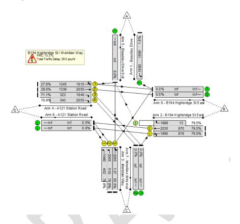
**Evaluation:** With extensive approach arm widening, access restrictions and possible carriageway realignment, modelling suggests that the signalised junction could operate within capacity under the 2036 scenarios tested.
