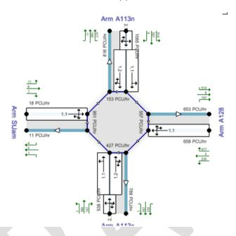
**Evaluation:** Located in a built-up residential area, there is little land available around the junction within which to expand the junction. Consequently, the proposed length of the approach arm widening, and the size of the proposed roundabout itself, would appear to be sufficient only to keep the junction operating within capacity in 2036 with the low growth scenarios modelled.
